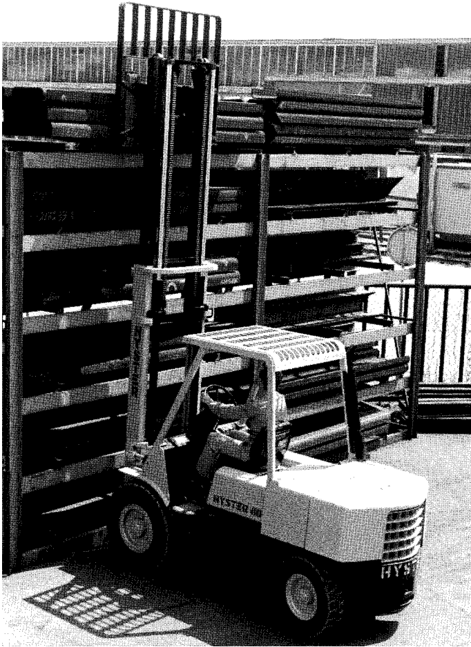
Figure 4.3.15 High lift fork truck with load rest, overhead and rear guards. (Courtesy Hyster Europe Ltd)
