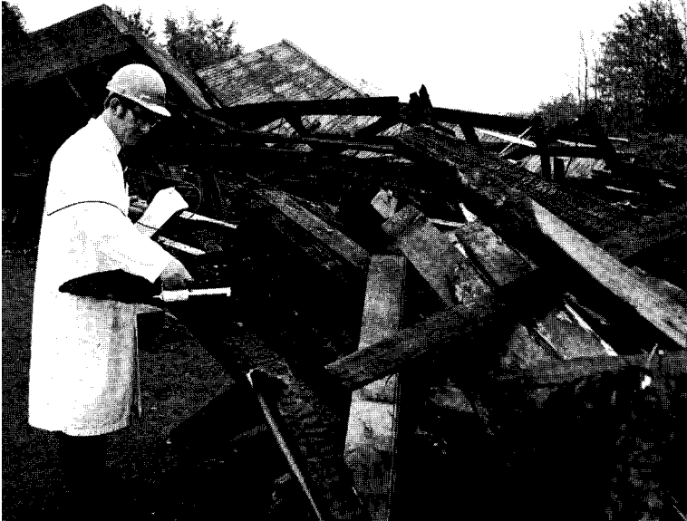
Figure 3.4.3 Checking contamination levels after a fire
